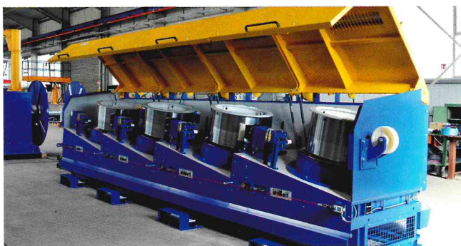
Individually configurable Straight-line drawing machine with 4 drafts Type 16/4 for maximum dimensional accuracy and reproducible quality. © VWP Maschinenbau- und Service
